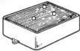
Cope after ramming with sand and removing pattern, sprue, and risers
