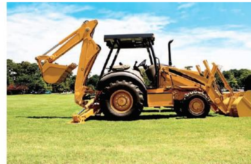
FIGURE 1-6 Construction backhoe and front-end loader (Shutterstock)
