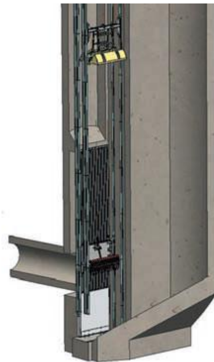
(b) Interior of lower shaft showing raker and clamshell
